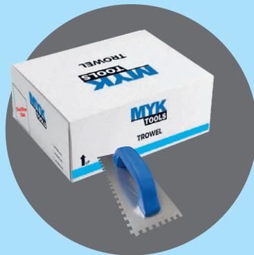
The notch trowel is great for professional tile / stone installations and multi-use, DIY renovation projects etc. It is used to create uniform bed thickness of tile adhesive to ensure complete adhesion of tile to substrate by reducing air pockets under the tiles.
