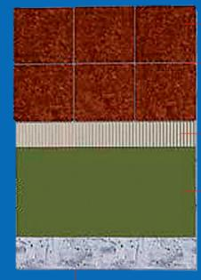
Properly Prepared Concrete, Backer Board or Masonry Substrates.
