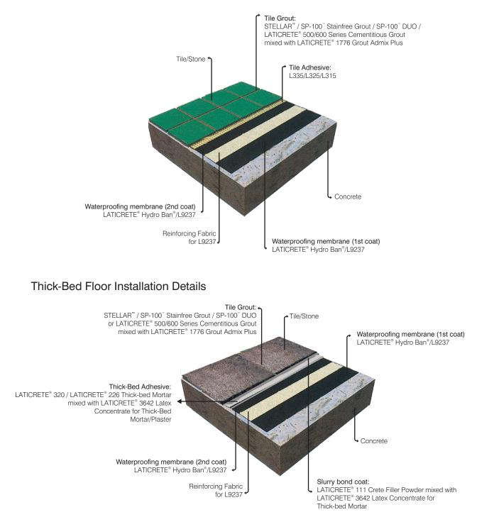
Note: LATICRETE® Hydro Ban® does not require use of Reinforcing Fabric, for crack bridging upto 3 mm
